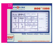
MOG1000. (PN 11391A70). Continuous flow neonatal emergency respirator. Ventilation Modes: CPAP, IPPV, SIMV with trigger.
